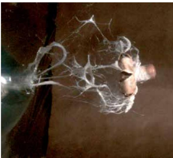
**EMB MONOBLOCK** controlled deformation bullet: on soft targets the outer annulus is deformed, increasing the area of impact without fragmenting and allowing the maximum possible energy to be released to the target. On reinforced or protected targets its harder central core has a good perforation capacity, keeping the necessary lethal energy.
